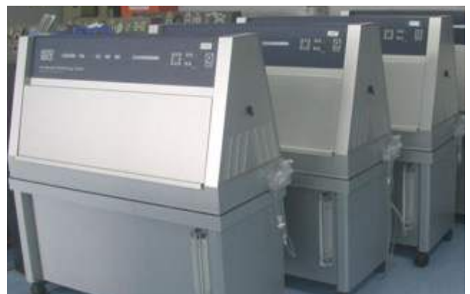
Figure 2: Hot QUVA with Solar Eye technology – used to test accelerated rates of weathering.
