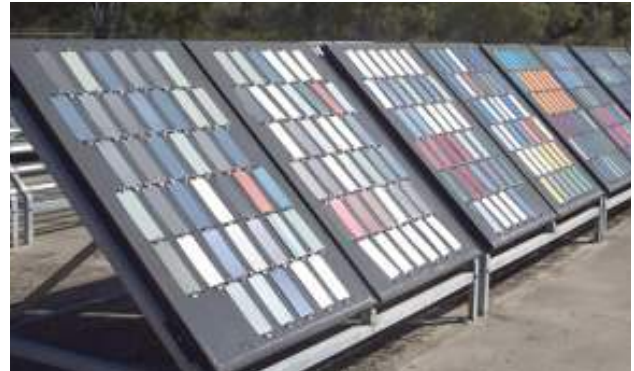
Figure 1: Outdoor Exposure – Hotracks, Rockhampton, QLD.
